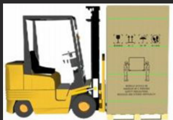
Figure 7 Please note the protection of module and forks
