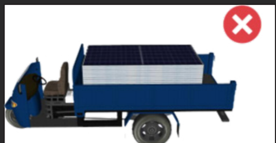
Figure 10 Do not use a tricycle to transport the Module
