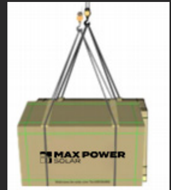
Figure 6 Schematic diagram of module lifting
